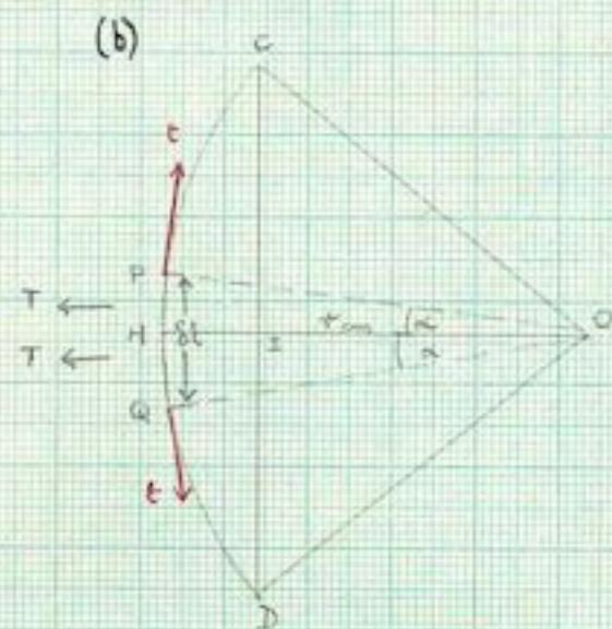
THEORY: Let the vertical sides of the thread be pulled into arcs of radius of curvature  $r$  cms. Let the tension in the thread be  $t$  dynes and the Surface Tension of the Soap Film  $T$ .
